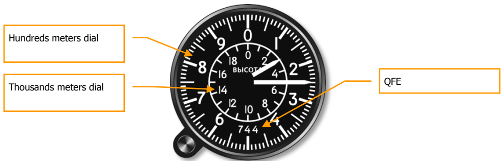
Figure 26: Pressure altimeter
