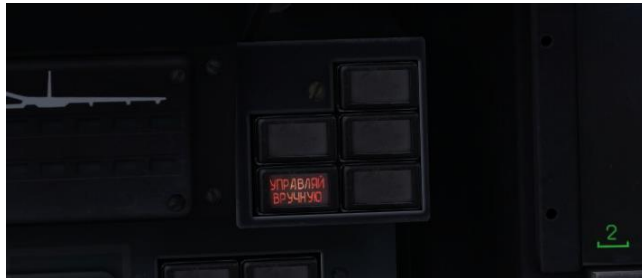
Figure 42: Manual Control annunciator
