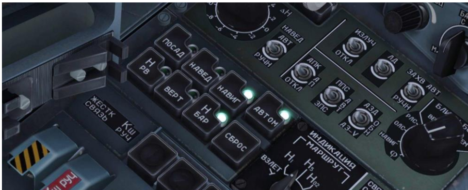
Figure 43: ACS push-light switches
