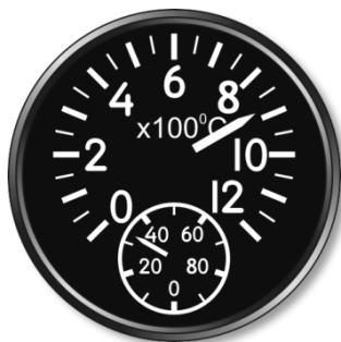
Figure 36: Interstage turbine temperature indicators
