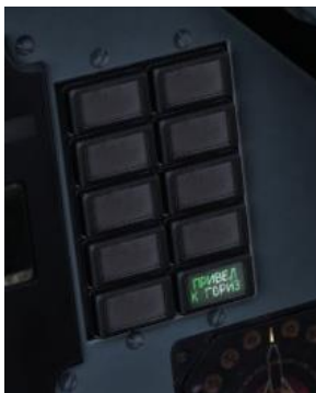
Figure 44: "ПРИВЕД К ГОРИЗ" (Level up to the horizon) annunciator
